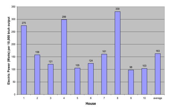
Chart #5: Loop Pump Electrical Power Draw per 10,000 Btuh of Heat Pump Output (Heating Mode)
