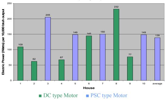
Chart #6: Blower Motor Electrical Power Draw per 10,000 Btuh of Heat Pump Output (Heating Mode)
