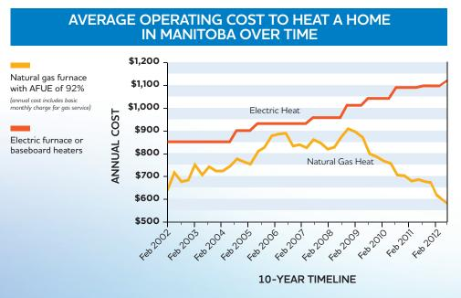
This chart compares the cost of heating the average home in Manitoba using natural gas (orange line) or electricity (red line). The costs are based on the rates in effect over the last 10 years.
