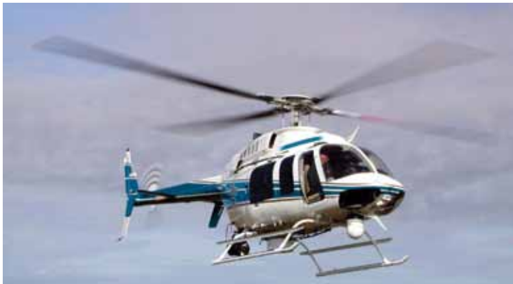
Through helicopters equipped with LiDAR scanning technology, WIRE Services collects a variety of data on transmission lines.
