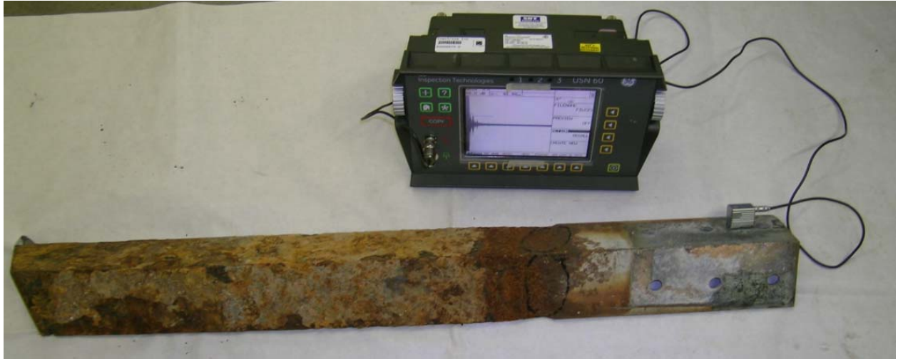
Figure 48 Setup of UT guided wave testing technique for inspection of tower leg samples.
