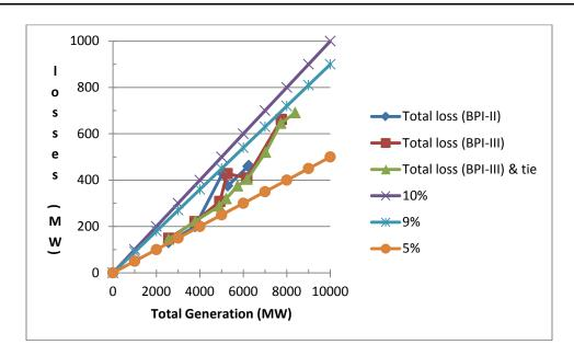
The expected losses ranged between five and nine percent of total generation. In the NFAT analysis Manitoba Hydro has made a conservative assumption of 10%. This value is reasonable for both the existing system and the future system including Bipole III and the new 500 kV tie to the U.S.
