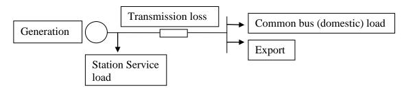
Assuming transmission loss is represented by an equivalent resistance (R), then  $I_{cb}^2R = Loss_{cb}$ . Transmission losses associated with supplying the common bus load is (Loss<sub>cb</sub>). Similar formulas can be derived for transmission losses associated with exports (Loss<sub>export</sub>) and total losses (Loss<sub>total</sub>).
