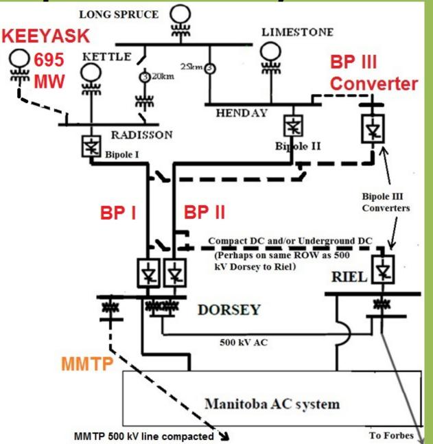
**Connect BP III** converter to the existing BP I or **BP II overhead** transmission lines – each rated at 3800 MW and used at 2000 MW can easily carry extra 695 MW
